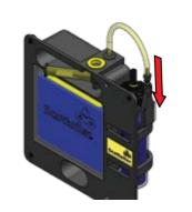
Connect the yellow siphon tubing to the filler plug luer. Insert filler plug into the primary reservoir.
