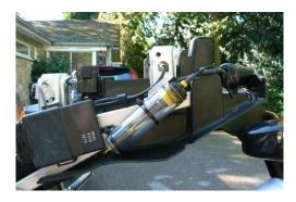
The Dispenser Assembly can be secured to the chain guard bolt using a Small Dispenser Plate & Clip. The delivery tubing can be routed along the chain guard using cable ties and glue or self adhesive cable clips. For further information see our easy step installation guide - Dispenser Assemblies, General. The nib should feed the rear sprocket between the 6 & 7 o'clock positions, with the cut face outwards. See picture bottom left
