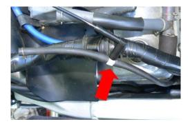
The RMV can be mounted to the frame. The more vertical the RMV the better and remember to avoid exhaust and engine components. For further information, see our easy step installation guide – Resrvoir Positions, General.
