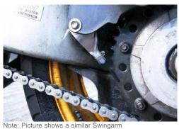
Once fitted, <u>fill and prime</u> the system and set the adjuster knob to 'prime'. Start the engine and turn the adjuster knob until a flow of between 1 and 2 drops per minute is achieved. Check the condition of your chain after a ride, and then adjust as required.
