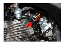
The RMV can be mounted on the frame or under the seat. The more vertical the RMV the better and remember to avoid exhaust and engine components. For further information, see our easy step installation guide – Reservoir Positions, General.
