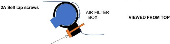
2x long self- tapping screws 3mm x 35mm through the carrier fixing into the air filter box. **2B Set screws**
