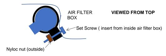
2 x M3 set screws about 40mm long and secured on the outside using 2 M3 nyloc nuts
