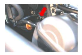
The RMV can be mounted under the seat, or behind the number plate. The more vertical the RMV the better and remember to avoid exhaust and engine components. For further information, see our easy step installation guide – Reservoir Positions, General. See third picture
