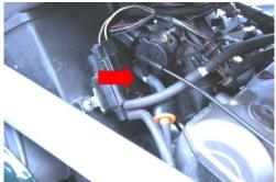
Note: Cut into the engine side of the check valve
