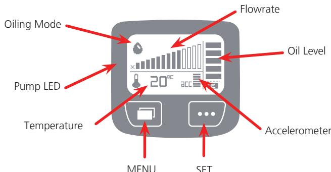
**Flowrate:** The flow rate is represented as bar graphs. The flow rate can be adjusted from 1 drop every 5 mins (slowest setting) all the way to 1 drop every .20 seconds (fastest setting). Pressing **SET** will cycle through the flow rates.
