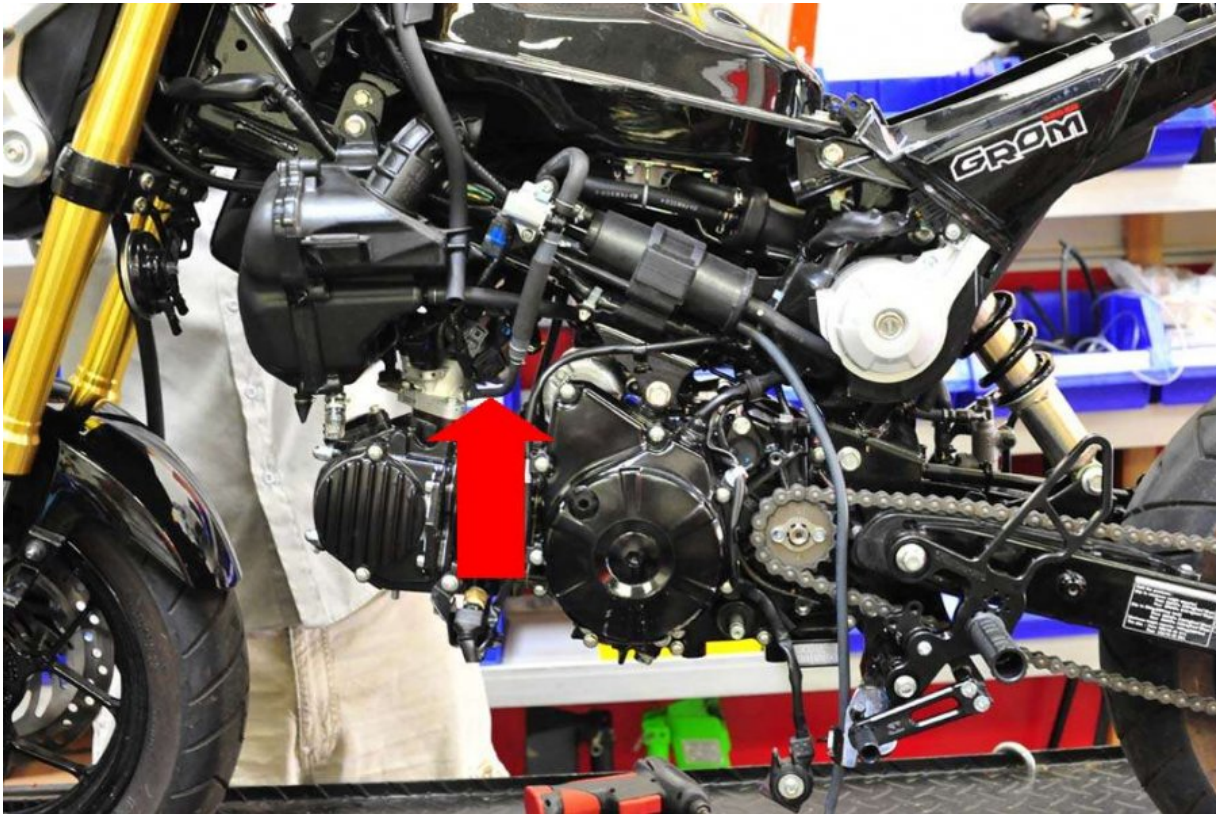
Vacuum pipe arrowed at throttle body.
