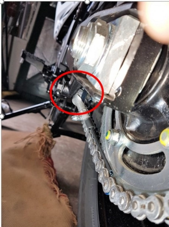
Attachment of delivery tube at rear sprocket
