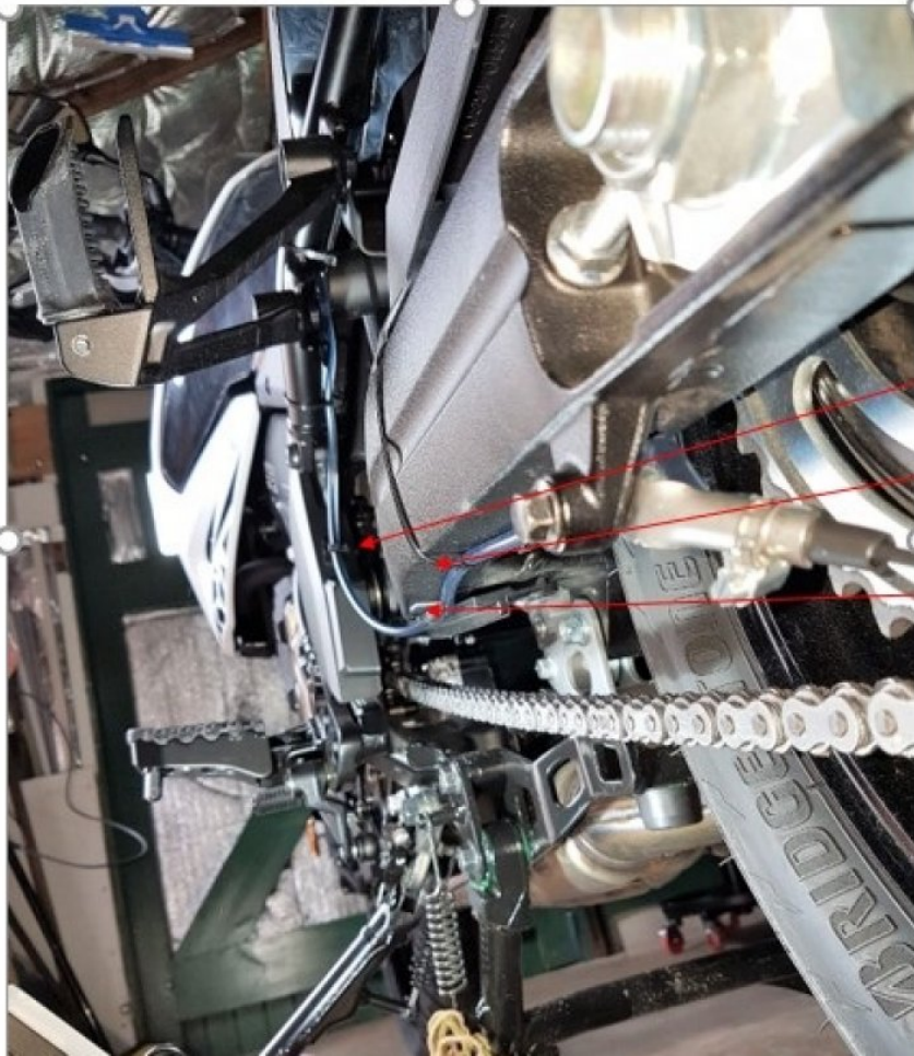
Routing of delivery tube #1 – under LH swingarm
