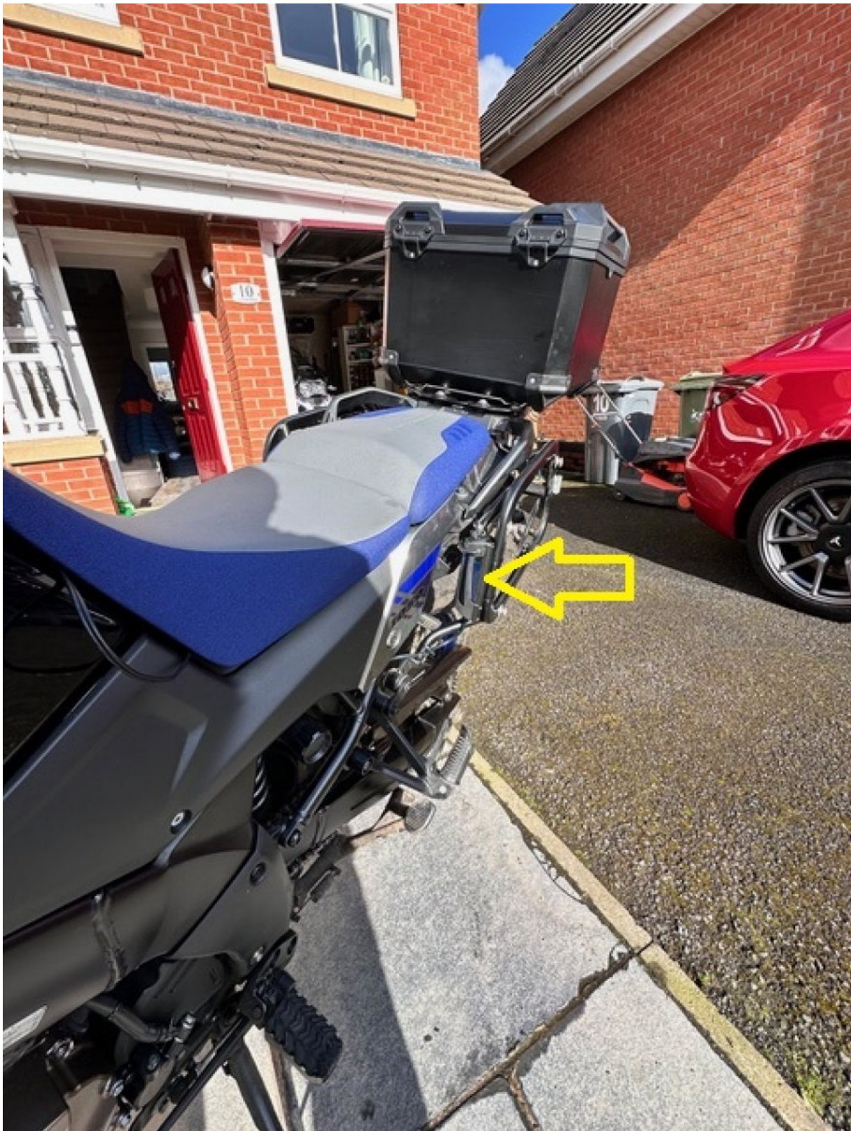
xSystem fitted onto the pannier rail
