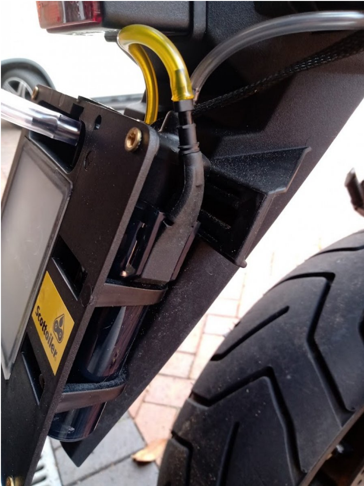
System fitted with HCR (High Capacity Reservoir).
