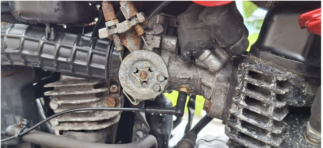
Spigot installed into inlet manifold.
