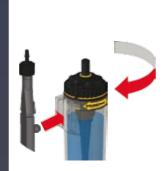
If the delivery tubing is empty:-Remove filler plug and breather from RMV. Using the new filler plug in the Lube Tube kit, press it into the side of the RMV. and set RMV to Prime.
