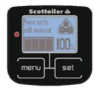
When an additional reservoir is in place the oil level gauge will display the overall capacity of the system.
