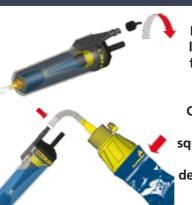
Remove twist lock connector from filler plug.
