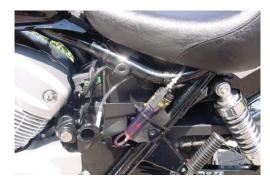
The delivery tubing can be routed along the swingarm using conduit and glue or self adhesive cable clips and the dispenser can be secured on the rear spindle using a Dispenser plate & Clip. For further information see our easy step installation guide - <u>Dispenser Assemblies</u>, <u>General</u>. The nib should feed the rear sprocket between the 6 & 7 o'clock positions, with the cut face outwards.
