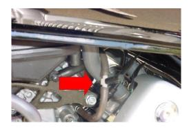
The RMV can be mounted under the seat. The more vertical the RMV the better and remember to avoid exhaust and engine components. For further information, see our easy step installation guide – Reservoir Positions, General.
