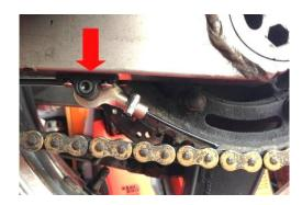
The REP can be mounted under the seat, or behind the number plate. The REP can be orientated anywhere between horizontal and vertical, as long as the nozzle is inclined upwards. Remember to avoid exhaust and engine components and to keep the filling hole accessible. For further information, see our easy step installation guide – Reservoir Positions, General.
